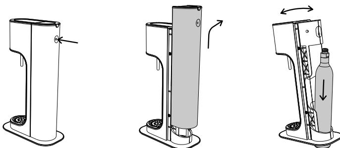
Tilt the sparkling water maker forwards and insert the gas cylinder through the opening in the bottom of the machine so that the cylinder is standing on the work surface. Gently tilt the sparkling water maker back so that the upper part of the machine rests against the threaded neck of the cylinder.
