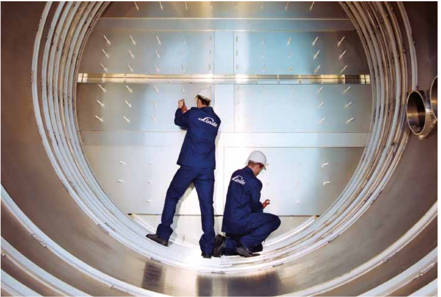
Fabrication of sieve tray column.
