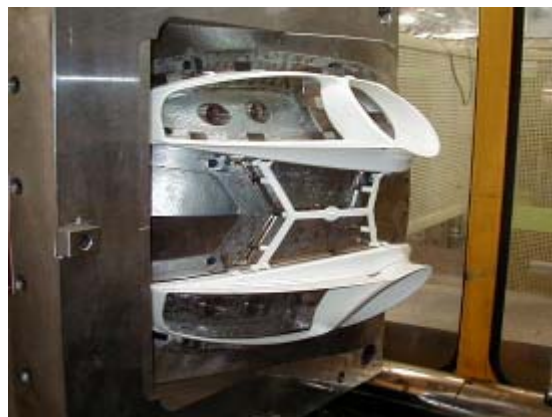
Reflector Housing in the mould (2 cavities)
